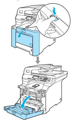
3 Hold the green handle of the drum unit. Lift the drum unit up and then pull it out until it stops.
